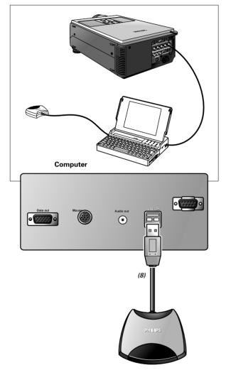
• Connect the supplied USB mouse receiver to the corresponding USB terminal on the PC.
